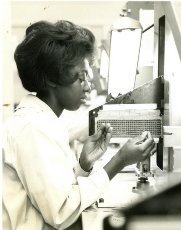
1969: 'Space age needleworker "weaves" core rope memory for [Apollo missions'] computers.' (Raytheon, 1969, p. 18)
